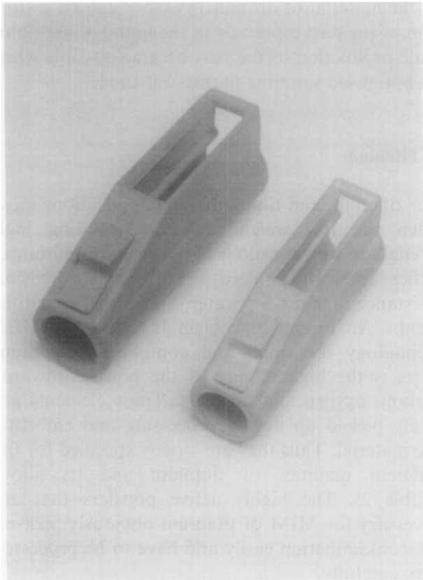
Fig. 9. W-Fe-Ni radiation shield, courtesy Advanced Technology Projects, ATP, Freilassing, Germany; left, green part; right, sintered part.
